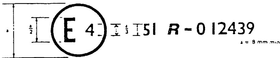
The above approval mark affixed to a vehicle shows that the vehicle type concerned has, with regard to its noise emission, been approved in the Netherlands (E 4) pursuant to Regulation No. 51 under approval No. 012439. The first two digits of the approval number indicate that Regulation No. 51 already included the 01 series of amendments when the approval was granted.
